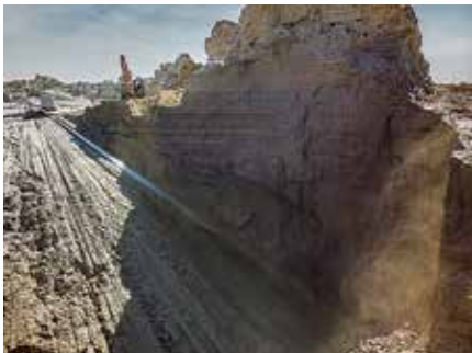
↑ Reclamation of tailings from the Driefontein 5 Tailings Facility by a remotely operated high-pressure water jet, ahead of retreatment at Far West Gold Recoveries' DP2 plant to extract gold
