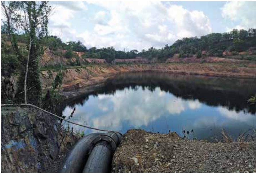
↑ Dewatering the satellite pit
