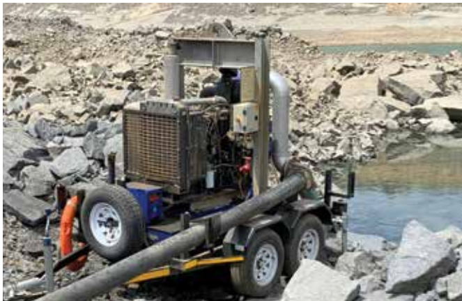
↑ The Sykes CP units weigh about 1.5 t on a road trailer, which allows easy mobility on-road and off-road
