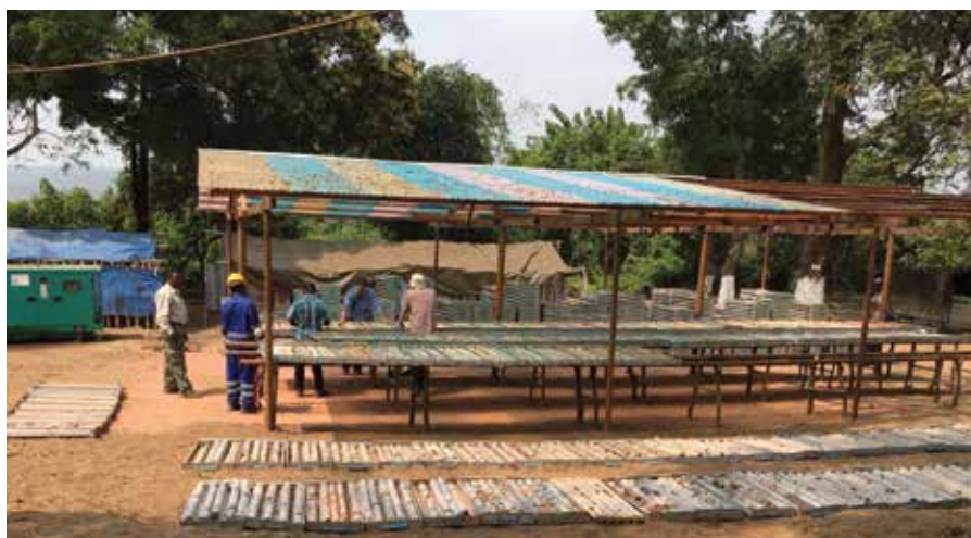
↑ Core sampling on site
