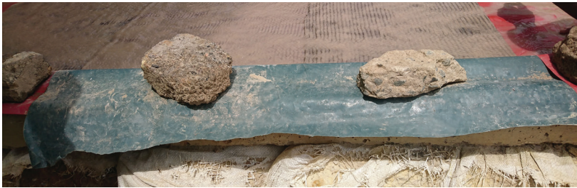
↑ A self-made drainage system to allow gold particles to be separated from sand
